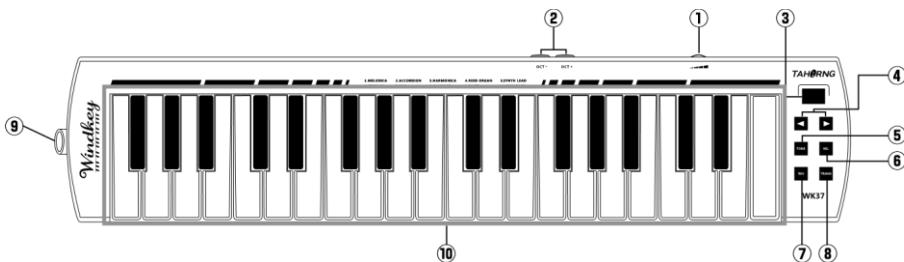
① Volume Wheel : This wheel adjusts the volume of Windkey. Turning it clockwise increases the volume.
